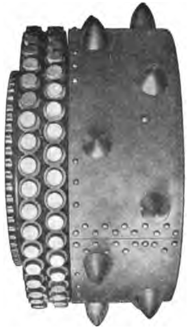
Fig. 3—Flat steel extension rims with heart shaped lugs: The 6 inch pair of these rims placed on the rear wheels increases the face of each wheel to 12 inches; the 12 inch pair increases the face to 18 inches.
