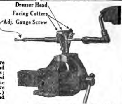
Fig. 5.—Illustrating the method for refacing a valve with a Healy refacing tool.
