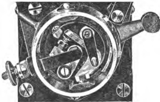
Fig. 2—Photographic view of the circuit-breaker or interrupter, on the opposite end to collector ring. Same type as shown in fig. 2, page 270, except interrupter arm above revolves clock-wise and fig. 2, page 268 revolves anti-clockwise.
