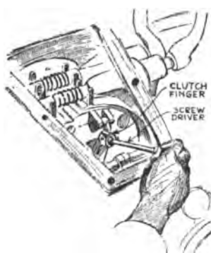
Fig. 15: Adjusting clutch fingers. Jack one rear wheel up, turn engine so clutch fingers come in convenient position, remove split-pin, give half a turn clockwise to the screw, and replace pin. Don't drop pins in transmission case. After long wear, new discs will be needed. It will be necessary to remove the transmission cover.
