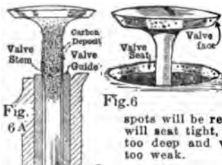
Fig. 6—Note the black spots on valve face and valve seat. This permits the escape of gas. If ground or re-seated the spots will be removed and valve will seat tight, if pitting is not too deep and valve spring not too weak.
