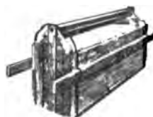
Fig. 24.—Crating a battery for shipment; note shape in illustration. Inside dia. should be 2" larger than battery and stuffed with excelsior. Label "handle with care—ACID."
