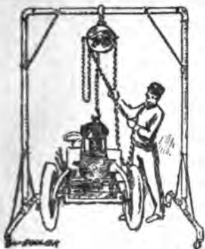
Fig. 4—A chain hoist and frame as shown above is a necessity in a repair shop for lifting engines from chassis. The frame is made of heavy iron pipe with rollers, also see other charts under "Repair Shop Hints," Inst. 46-D.
