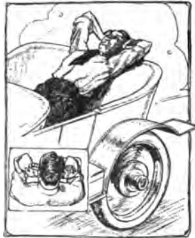
Fig. 1—Listening for rear axle hums; the hands are placed in front of the ears to intercept the sounds
