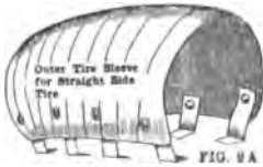
Figs. 9, 9A—Outer shoe, to be placed temporarily on outside of tire when cut or damaged until vulcanized. Note lower part fits under rim for clincher, and under tire for straight side.
