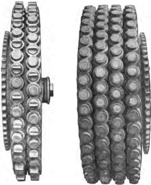
Fig. 4—Wood plug extension rims are made in either a one or two row wood plug extension rim. The single row rim increases the width of the wheel to 9 inches and the double row to 12 inches.
