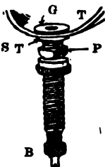
Fig. 2—The old style double tube clincher bead tire on a one piece clincher rim. Note the lug formerly used to hold tire on the rim. Pneumatic tires were called "double tube" tires in the early days to distinguish them from the single tube tire, fig. 1.
