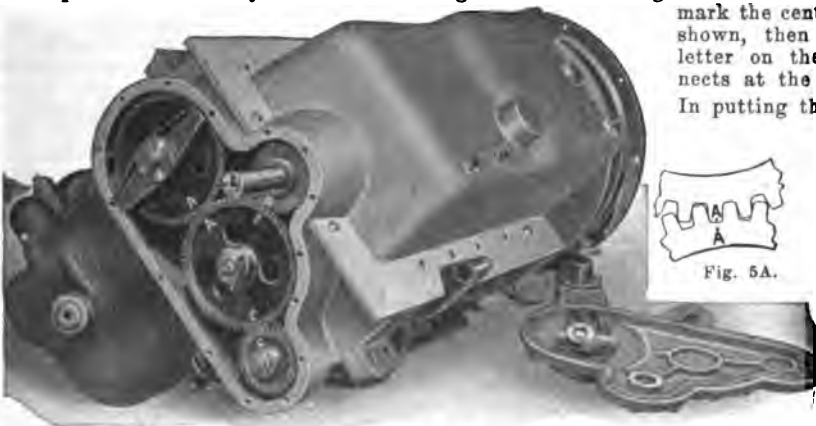
Fig. 5—Showing how the gears are arranged. O—drives the magneto and circulating pump; next gear to it is idler gear, placed between the small crankshaft gear B and O; the gear on which governor is attached is the gear which drives the cam shaft and oil pump and is driven by the idler gear also. Therefore cam shaft gear revolves \frac{1}{2} the speed of crank shaft gear.
