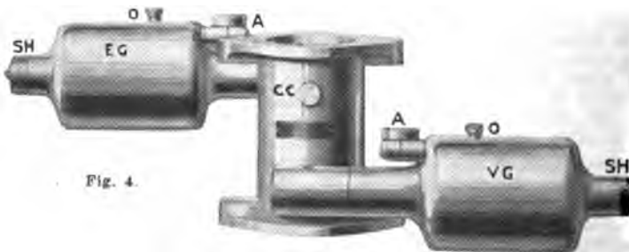
Fig. 4—Pierce dual purpose governor. EG—engine governor; VG—vehicle governor; CC—connects between carburetor and inlet manifold; SH—where driving shafts connect; O—oil cups; A—adjusting screws and seals.
