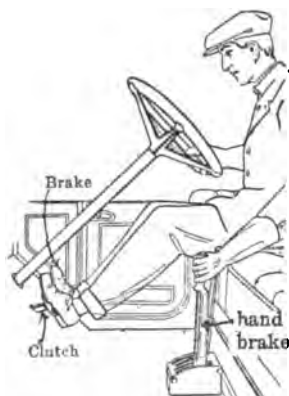
Fig. 1. See that gear shift lever is in "neutral" before starting. Release hand brake, then throw clutch "out."
