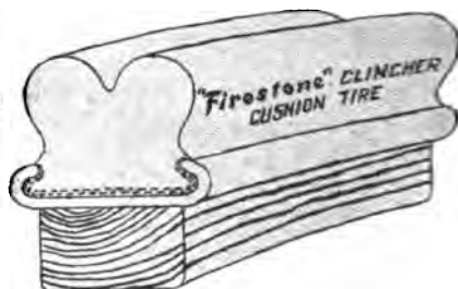
Fig. 5.—Firestone clincher cushion tire interchangeable with pneumatic tires on regular clincher rims.
