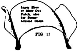
Fig. 11—Inner shoe, to go on inside of tire to protect fabric cuts, breaks or weak places due to small blow outs or stone-bruises or rough spots and also a protection to rim cuts. Made of 3-ply fabric with wings, to go under the rim.
