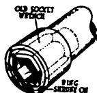
*Fig. 1—Extension socket wrench: By mounting a socket wrench head in the end of a 4 ft. length of 3-inch pipe, an extension wrench is made that facilitates the removal or replacement of the nut on the rear axle drive pinion. A steel ring is first shrunk on the end
