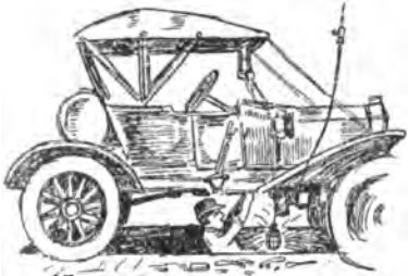
Fig. 1—A pit is provided in most shops. The car is rolled over the pit. Size of pit is usually 6 ft. long, 2 ft. 9 in. wide and 2 ft. 9 in. deep. A very well laid out plan for a pit is shown in chart 244-A.
