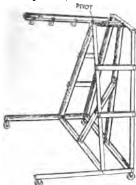
Fig. 4—A chain hoist and frame as shown above is a necessity in a repair shop for lifting engines from chassis. The frame is made of heavy iron pipe with rollers, also see other charts under "Repair Shop Hints," Inst. 46-D.
