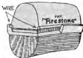
Fig. 1.—Side wire solid tire. The original automobile tire, now used on light trucks, trailers, cabs, horse-drawn vehicles, etc.
