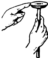
Fig. 4—Smear the valve grinding compound around edge of valve.
