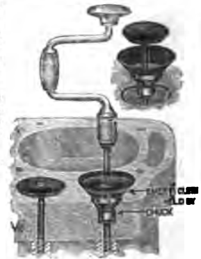
Fig. 8.—McCullough valve reseating tool consists of a carborundum cloth cone held to the face of the valve as shown. The valve is used just the same as a reamer. The cloth cutting the seat in the cylinder exactly the same bevel as that of the valve face. No reamers are required. There is nothing to replace but the carborundum cloth. Emery cloth or sand paper will do quite as well but will not last as long.
