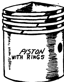
Fig. 9.—In order to prevent compression passing through joints of rings; they are placed as illustrated. Three rings is the usual number to a piston.
