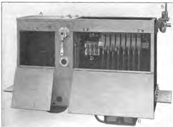
Fig. 4: Controller box. A—sheet steel controller box; B—controller handle; C—three way switch; D—lamp circuit fuses; E—plug for portable lamp; F—resistance.
