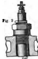
Fig. 2: Recess around plug shell retains heat.
