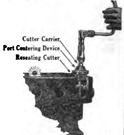
Fig. 6.—Illustrating the method of truing up a valve seat and reaming a worn valve stem guide.
