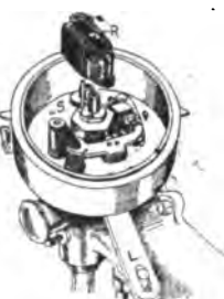
Fig. 3—Breaker and distributor mechanism. The brush is readily removed
