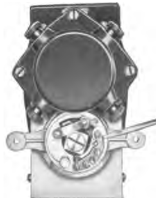
Fig. 33—Showing method of raising or lowering platinum point screw in (6) fig. 40. The usual distance to set these points are .020 or \frac{1}{64} ". This adjustment can be made with a screw driver. Spark plug gap is set .025.
