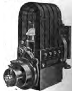
Magneto and lubricating side: M—magneto, K. W. high tension; S—shaft driving magneto, which is driven by gear in gear case (H); O—force feed lubricator driven by belt (B)—see page 195 for the "mechanical type"; P—water pump; E—breather pipe; Y—hand hole plates to reach bearings, and through which pistons and connecting rods can be removed; G—governor, "fly ball" or "centrifugal" type.
