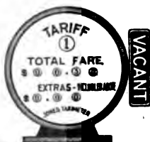
Fig. 2 — Taximeter starting with tariff sign showing one fare or passenger.
