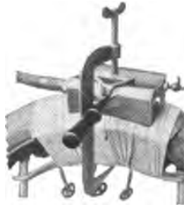
Fig. 26. Apply heat to inside and outside simultaneously.
