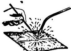
Fig. 22. Incorrect method of applying filling material. The blow-pipe is also held at the wrong angle with relation to line of weld.
