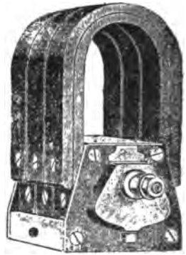
Fig. 3—The low tension magneto complete. View shows the drive end of the armature, which is driven at a fixed speed from crank shaft of engine, by gear or chains. The armature has one winding.
