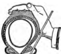
Fig. 1—The First Operation in removing a tire cover: After the lug bolts wing nuts have been slackened off, the edge of cover is pushed out of the rim and the tire levers inserted. Various forms of levers are obtainable, some being more convenient to use than others. Most of the tire makers supply suitable levers for their tires.
