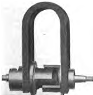
Fig. 31—Rotating poles on the Dixie model 120—for 8 and 12 cyl. engines. Note there are 4 rotating poles. On the 4 and 6 cyl. there are 2.
