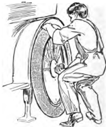
Fig. 4—Testing rear wheel bearings: Lost motion in a rear wheel bearing is best tested for by taking hold of the tire with one hand to steady the body, then working the wheel up and down with the other hand, assisted by the knee and lower portion of one leg. When the right hand is placed on the hub, the right leg is often more conveniently used than the left, as shown in the illustration.
