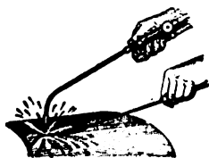
Fig. 21. Correct method of holding the blow-pipe with relation to the line of weld.
