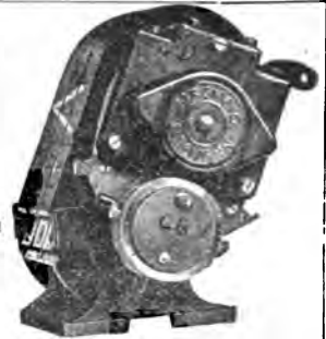
Fig. 3.—The Eisemann high tension magneto, pivoting or rocking advance magneto. The advance and retard is obtained by rocking the magneto bodily on its cradle. Otherwise the magneto is the same as other magnetos. Armature revolves.
