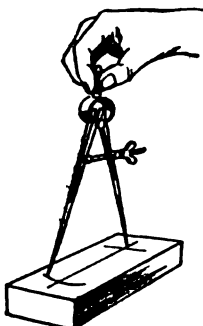
Accurately mark off the center distances with a pair of steel dividers, after first lightly pre-punching one center
