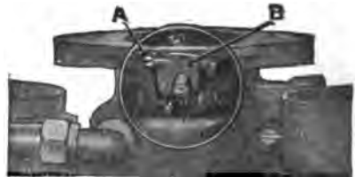
A.—Stop arm screw. B.—Stop arm. Turn screw A to left to throttle engine lower.
