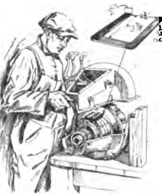
Fig. 16: This clamp is used to hold transmission bands together while replacing the transmission cover. It is made of spring steel \frac{1}{2} in. wide and \frac{3}{32} in. thick, bent into the form of a U, having legs 3\frac{3}{4} in. long and being 2\frac{1}{16} in. across. One of these is clamped over the lugs on the transmission bands before replacing the cover and removed after the cover is bolted on. (Motor World.)
