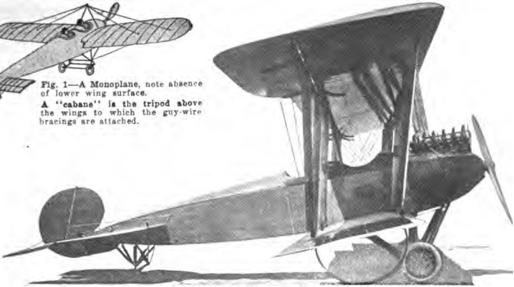
Fig. 2—A modern tractor type Biplane. Equipped with Hall-Scott type A5 engine. Note the "cambered" wing and "staggered" struts.
