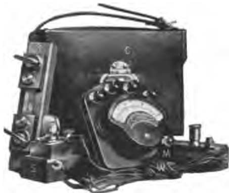
Fig. 1.—Weston Model 280 Combination Volt-ammeter (M) with case (C), three shunts (S), cables (W).
