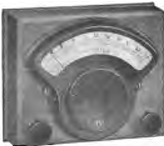
Type 515D Cadmium Voltmeter. Reads: .3-0-2.7 volts. The .3 reading is to the left of 0 and 2.7 to right of 0.
