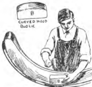
Easy method of removing dents from fenders with the use of a shaped wood block.
