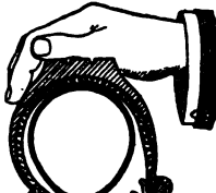
Fig. 3—Third Operation: The hand is used in assisting the working of cover down outside of the rim, the lever being in position between cover and rim. A new cover will generally be forced stiff to manipulate with the hands for the first time, but soon become supple with use.
