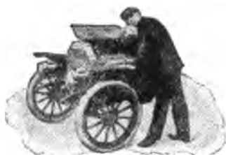
Detecting noise of engine by sound, with a Sonoscope. Same principle as sounding rod above. Made by American Elect. Co., Chicago.
