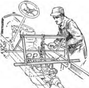
A suggestion for making a hoist to raise and lower transmissions where considerable of this work is being done.
