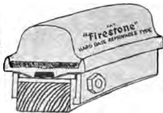
Fig. 3.—The hard base tire on removable rim.
