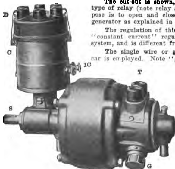
Fig. 2. Westinghouse generator with the ignition distributor and timer and high tension coil mounted on the generator. The coil is beneath the distributor and timer. The generator is driven by a silent chain from cam shaft, the distributor shaft is driven from a spiral gear on armature shaft (S), and is of course driven at cam shaft speed. T, generator terminals (see fig. 1, F-A); G, ground connection terminal.
