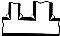
Fig. 35. Shows preparation of pipes before welding to form branches.
