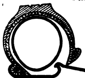
Fig. 4—Fourth Operation: The inner tube having been carefully replaced, the hooked end of the lever is used to work the edge of cover back into the rim.
