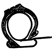
Fig. 2—Second Operation: The lever raising the cover over the edge of the rim. Special care must be taken not to pinch the air tube between rim and lever. This would result in damage to the tube, rendering it useless till repaired. Even if not cut through, the rubber would be so much weakened as to burst under the effect of air pressure some future occasion.
