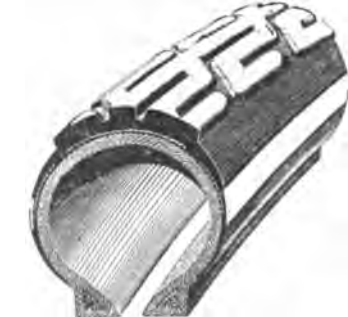
A straight side bead tire with a non-skid tread. Can be either the "fabric" or "cord" type of carcass, as explained on page 565.
