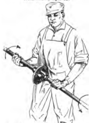
Fig. 7—in testing the adjustment of the differential gears, grasp the assembly in this manner, and turn the axle in opposite directions. They should turn freely all around.
