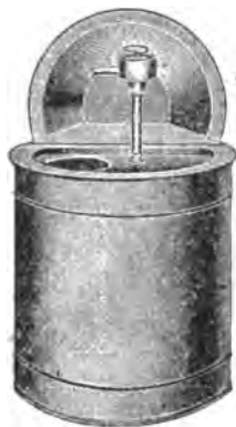
Fig. 1—Lubricating oil tank. This tank can be used for engine oil and general lubricating oil. It is made of galvanized steel and holds 60 gallons. Fitted with a positive action force pump. The advantage is that it keeps the oil covered and free from grit and dirt. The Bowser Co. of Ft. Wayne, Ind. make a more elaborate affair.
