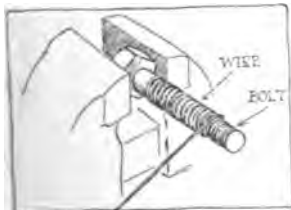
Fig. 4—How spring is made by winding wire around bolt
