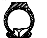
Fig. 6—Illustrating a serious fault. The inner tube has become slipped between one of the lug bolts and cover, and unless released will result in a burst tube. This risk is avoided by taking care to moderately inflate tube before replacing in cover.
